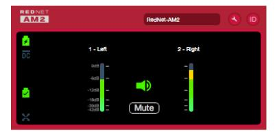
The illustration above shows a RedNet AM2 with the Line Out Mute inactive and shows signal present on both channels. It has PoE power available and has a locked network connection.
